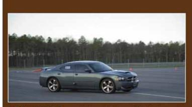
FOR COMPARISON, we rounded up a stock Charger R/T and ran it around the NJMS skidpad to a best of 0.87G. SRT8s are rated at 0.88G. Respectable, but there's definitely room for improvement.
