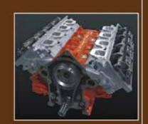
THE ARRINGTON Gen-III 420 Hemi starts life as a 6.1-liter factory suitable wall thickness before being bored and stroked to 426 cubes. A custom cam, head work, intake work, massive Arrington throttle body and a proprietary computer "tune" all work in harmony to develop the 600 horsepower. vet maintain a stock-like idle.
