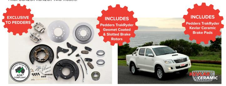
Independent Australian engineering test results proved that at 100kmh the TrakRyder rear disc braking system upgrade stopped 21.4m sooner than original equipment with just 30% braking force. An amazing result that enhances load carrying and towing performance.
