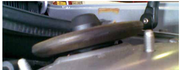
This worn top mount has come loose. This is a common fault once the unit has failed.
