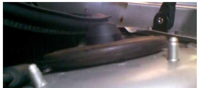
This is what a new top mount looks like once fitted. Pedders recommends the use and fitment of its 5030 and 5851 for the top mounts of Holden Commodore VR-VE models.
