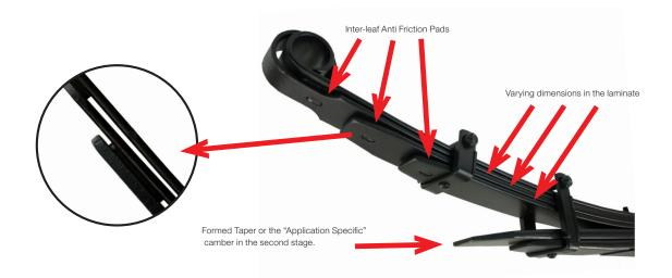
Inter leaf friction is created with the leaves flexing through normal suspension travel, as a consequence a firmer ride may be experienced. With the fitment of "Inter Leaf anti friction pads" this reduces the resistance to movement and therefore will improve the quality of ride.
