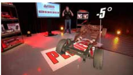
**5. Wheel Alignment:** This is the correct angle of a vehicles tyres to maximise tyre contact under normal driving conditions. Increased weight causing changes in suspension travel and geometry, which affects the angle of the wheel resulting in the reduction of tyre contact with the road and increased tyre wear. Incorrect Wheel Alignment and Tyre Contact affects all facets of vehicle performance, most importantly safety through diminished steering responsiveness and braking efficiency.
