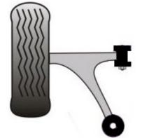
So remember, check all the bushes front and rear so the car maintains good steering, handling and extended tire life.
