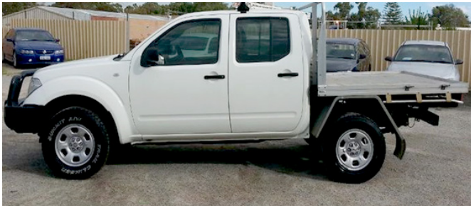
Correct length tray for the wheel base and load carrying capacity.
