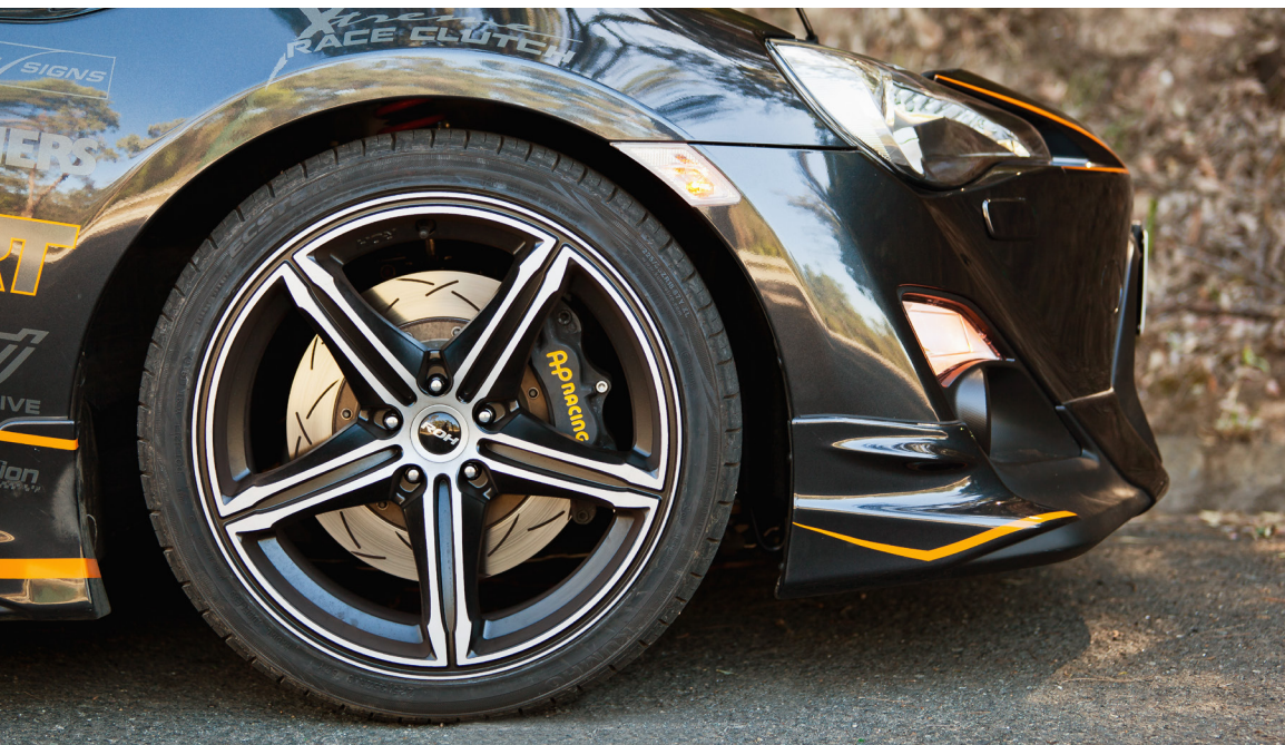
ROH's latest 'Arrow' design 18s look tough, but also allow space for massive 330mm two-piece rotors and four-pot AP calipers
