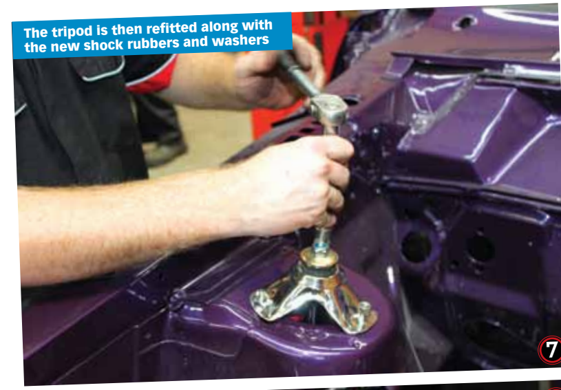
New spring saddles and Pedders 90/10 shocks were fitted. The springs are 6 cylinder versions to allow for maximum lift when drag racing with the sway bar removed
