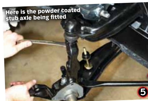
We used rubber bushed upper control arms as available on XA onwards Falcons. It basically means maintenance free operation and no squeaks
