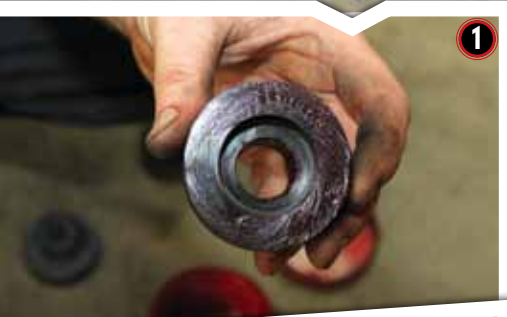
The radius rod bushes are greased up before being fitted
