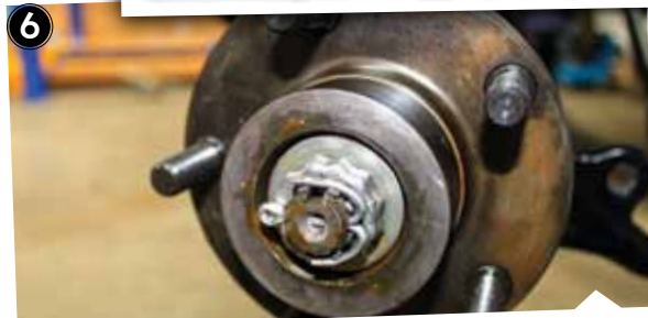
Refit the bearing tab washer and fit the centre nut tightening to the recommended preload. We tightened the nut tightly then backed it off half a turn. Over tightening will destroy the bearings easily. Don't forget the split pin for safety
