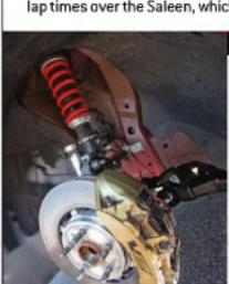
> The Camaro also runs Pedders adjustable coilovers on the front, with Cadillac CTS-V brakes swapped in. The Caddy front brake interchange is a relatively simple upgrade for the fifth-gen Camaro.
