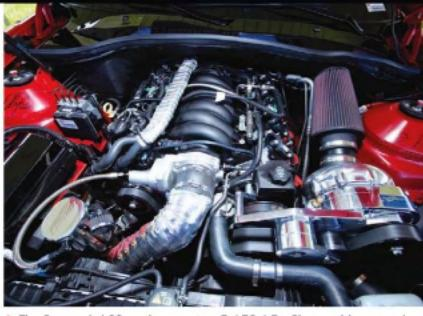
> The Camaro's LS3 engine sports a P-15C-1 ProCharger blower and Stage II intercooler system. On the Dynojet chassis dyno, it makes 556 hp and 481 lb-ft at the wheels. Pedders USA continues to work on managing the brute's air inlet temperatures.
