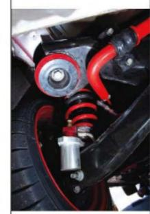
> Shown here is the Camaro's left rear corner with Pedders spring. shock, and fat antiroll bar. The big red doughnut at upper left is the Pedders subframe bushing insert.
