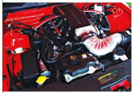
> The Mustang 4.6L V-8 employs Saleen's well-developed, OE-style supercharger and air/water intercooler. This setup produced 449 hp and 419 lb-ft on the chassis dyno. A special Saleen strut brace is required to clear the blower assembly.
