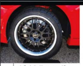
> Both the Mustang and Camaro run identical Bridgestone RE-11 305/30-19 tires front and rear on Forgeline 19x10.5 wheels. Special offsets were devised to fit the rubber inside the fenders and square the track widths, but you'll need to contact the Forgeline people for those specs. That's hard-won intellectual property in their book.
