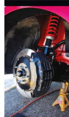
> The Saleen Mustang is equipped with Pedders USA's tasty coilover units with fully adjustable spring seats and dampers. The brakes are six-piston Saleen units, which according to John Buttermore, provide better feel at the limit than the Camaro's stoppers.
