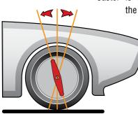
Caster is the angle between the steering axis and the vertical, viewed from the side of the car. Too much caster causes heavy steering. Too little caster makes the car 'wander'. A car will pull towards the side of the car with the least positive caster. Unequal casters can also cause braking problems on some vehicles.
