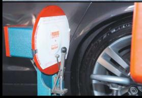
How well your car passes this test will be determined by the difference between each shock's maximum figure value, obtained during the test and a known standard: A Pedders shock absorber unit.
